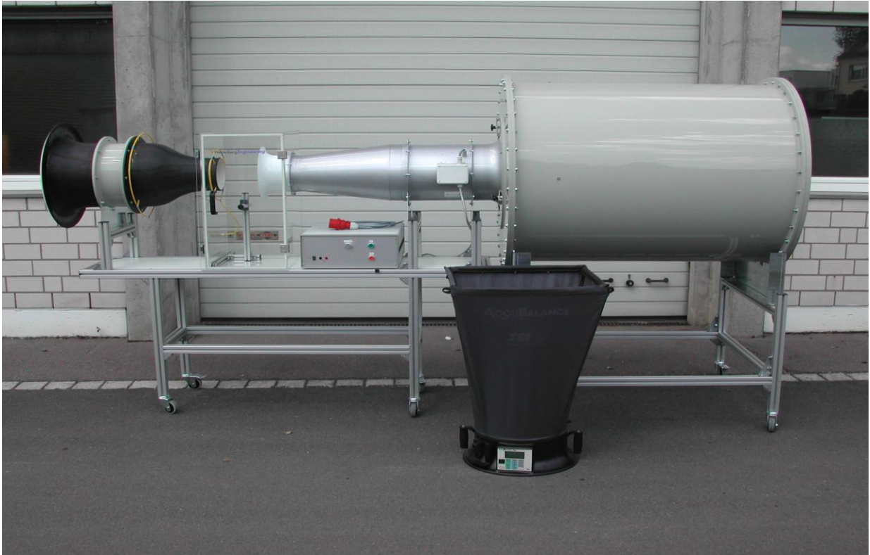
Fig. 2 Wind tunnel with extension module for air flow hoods
