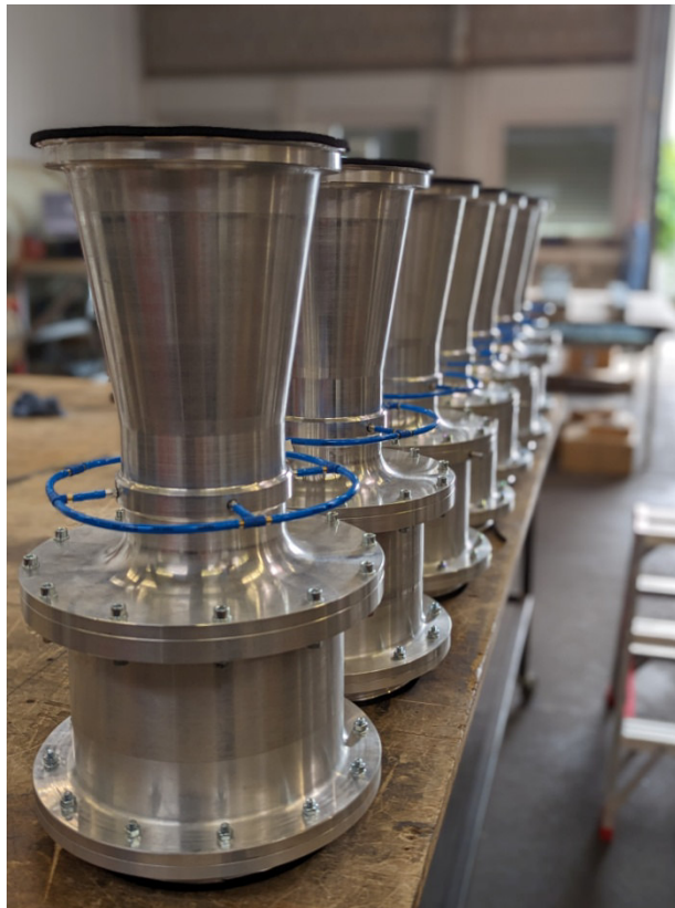
Fig. 1 Venturinozzle made of aluminum
