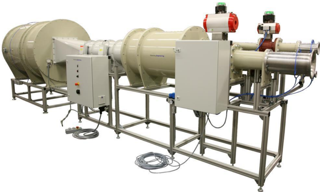
Fig. 1 Volume flow test bench
